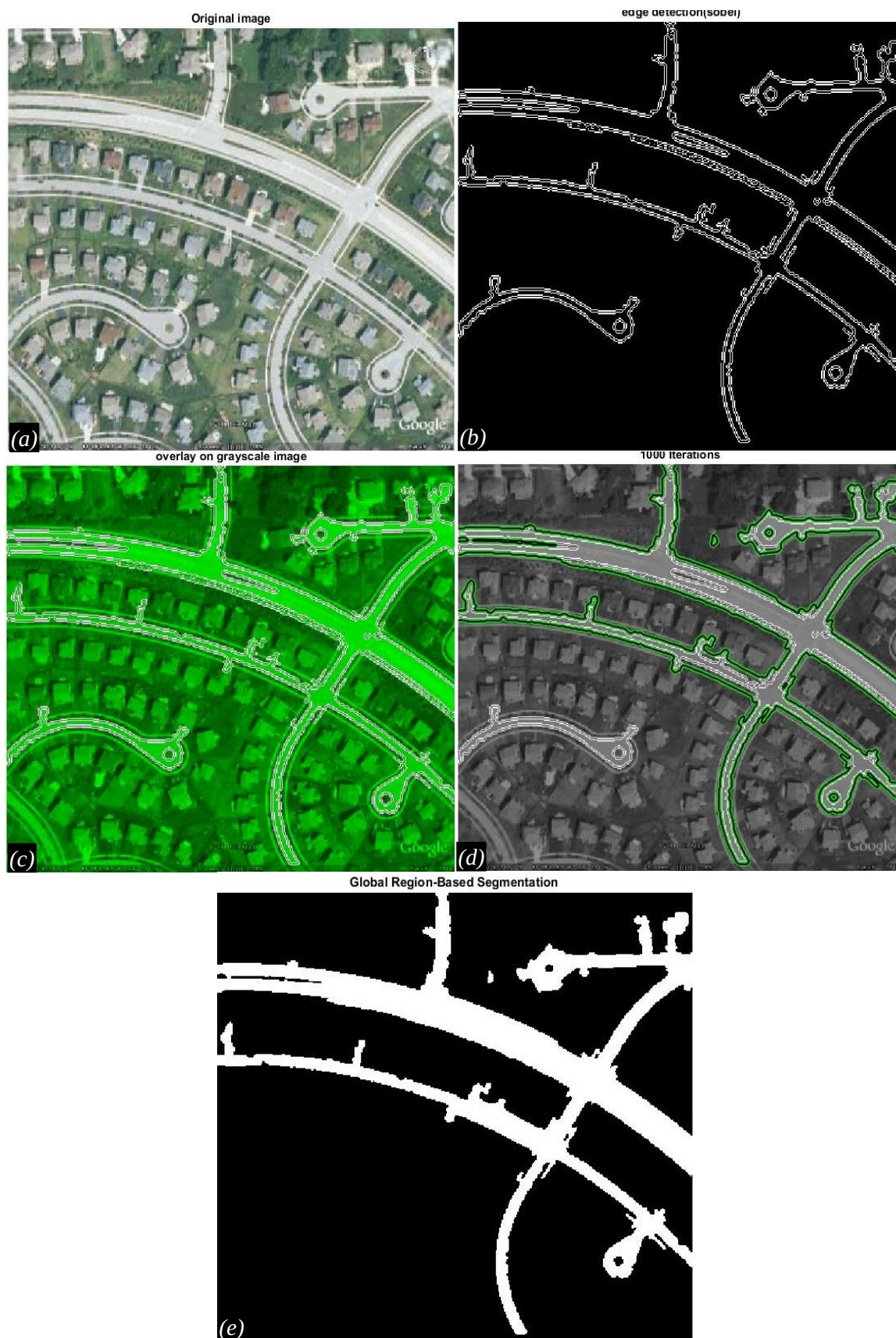
Fig. 1: Proposed Algorithm Applied on an Image with Developed Urban Area. (a). Original Image, (b). Final Edge Detected Image, (c). Merged (Original and Edge Detected), (d). Image with Active Contours, (e)Final Extraction of Road.
