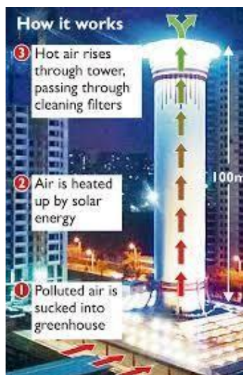
Figure 9. Mechanism of Air Purifier
